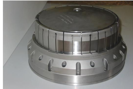
Expanding possibilities: Collet mandrel used for manufacture of precision large diameter bearings
