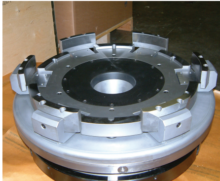
Getting a grip: Segmented diaphragm mandrel used for large gear manufacture
