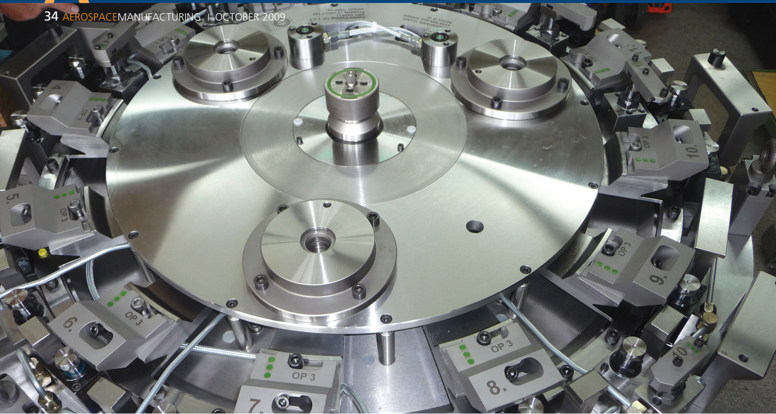
All shapes and sizes: Multi-segmented diaphragm membrane with swing clamps and work supports
