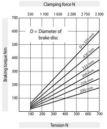
The braking torques shown in the diagram are based on a theoretical friction coefficient of 0,4.
