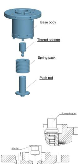
The spring force actuator for balancing machines consists of the base body, spring pack, push rod and thread adapter.
